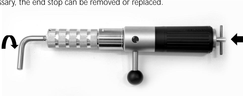
Clean the chuck, lightly grease it on the outside, and reinsert it in the shaft. Use the locking tool and the chuck key as described above to lightly tighten the chuck on the shaft. Replace the cable connector and secure it with the screw cap. Reinsert the milling spindle into the chuck.
