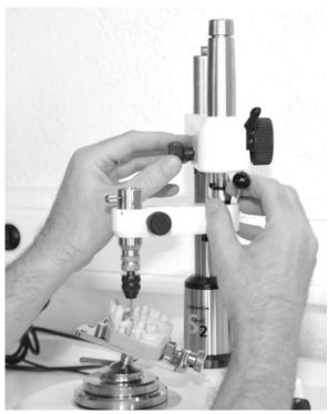
Thanks to the additional fixing screw on the milling arm, it is possible to arrest the arm in any extension position. This permits attachments to be mounted without problems.
